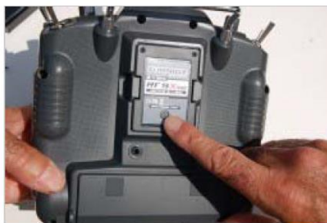
Insert the special cable (loop) in the file "BATTERY" and connect the receiver battery in position "BIND", wait until the LED flashes red.
