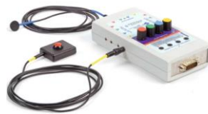
Figure 17: g.TRIGbox used to synchronize sounds and EEG acquisition.
