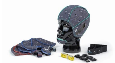
Figure 14: Scalp called g.GAMMAcap in where the electrodes are placed.
