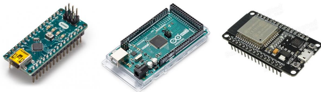
Figure 5.- From left to right: Arduino Nano ATmega328, Arduino Mega 2560 ATmega2560, and ESP32-DevKitC. (Arduino, n.d.; Espressif, n.d.)
