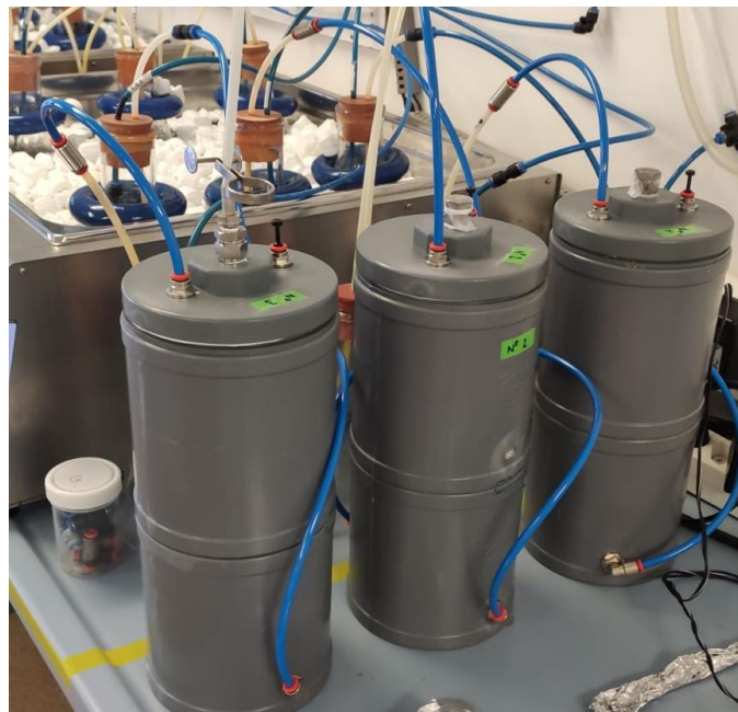
Figure 3.3 Bench-scale PVC reactors (not-isolated) used to perform SSF.
