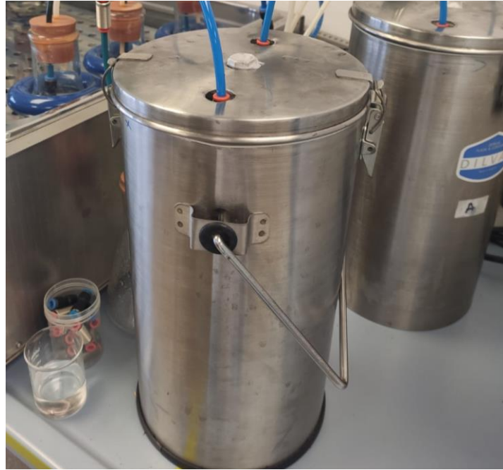
Figure 3.4 Bench-scale Dewars reactors (near-adiabatic reactors) used to perform SSF.
