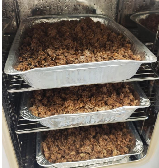
Figure 3.5 Tray-type reactors used to perform SSF.
