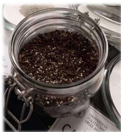
Figure 6-8. End product obtained from PS composting process amended with mesolite addition.
