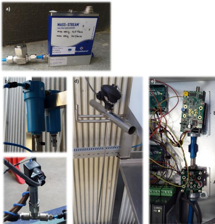
Figure 4-5. Monitoring and control devices of biodrying and composting systems developed.
