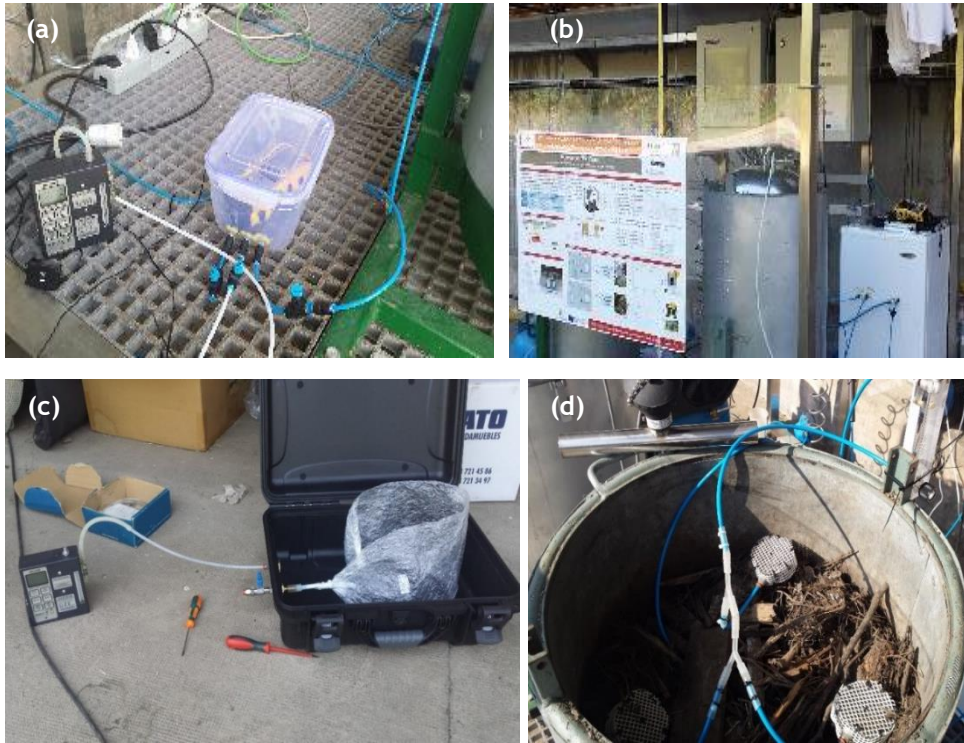
Figure 3-10. Sampling procedure of gaseous emissions: (a) sampling of NH 3 , tVOC and H 2 S emissions using a pump to dilute gaseous sample with external air, (b) semi-spherical stainless-steel flux chamber used for biodrying gaseous emissions sampling, (c) suction pump and hermetic box for biodrying gaseous emissions sampling (group 1), (d) gaseous emissions sampling device for biodrying samples (group 2).
