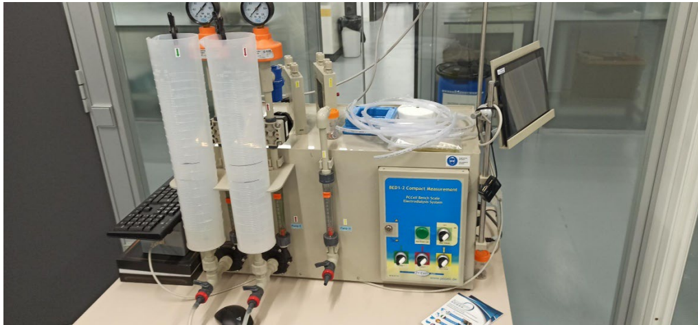
Figure 7.5. Electro dialysis equipment used as last step of water recovery system.
