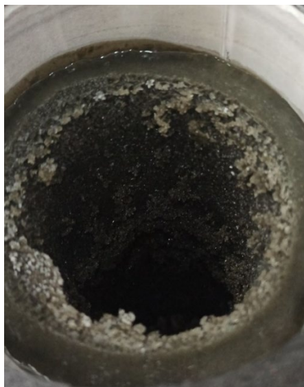
Figure 6.2. Formed ice during the PFC of PS before (A) and after vacuum application (B).
