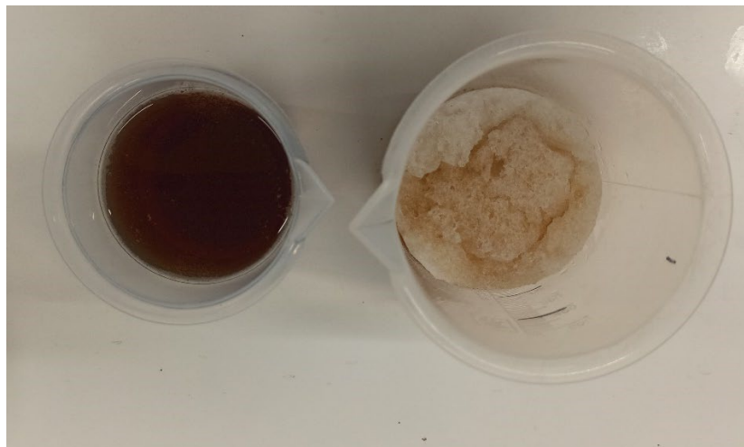
Figure 5.5. Concentrated and ice fractions obtained from the SFC of the RO concentrate separated through a vacuum suction stage.
