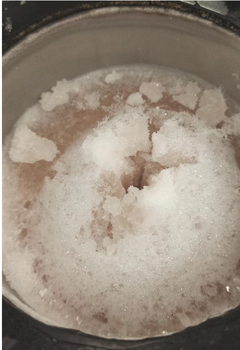
Figure 7.8. Structure of formed ice from studied brine solution when the salt concentration is low in S5 (A), and when the concentration of ice is high in S1 (B).
