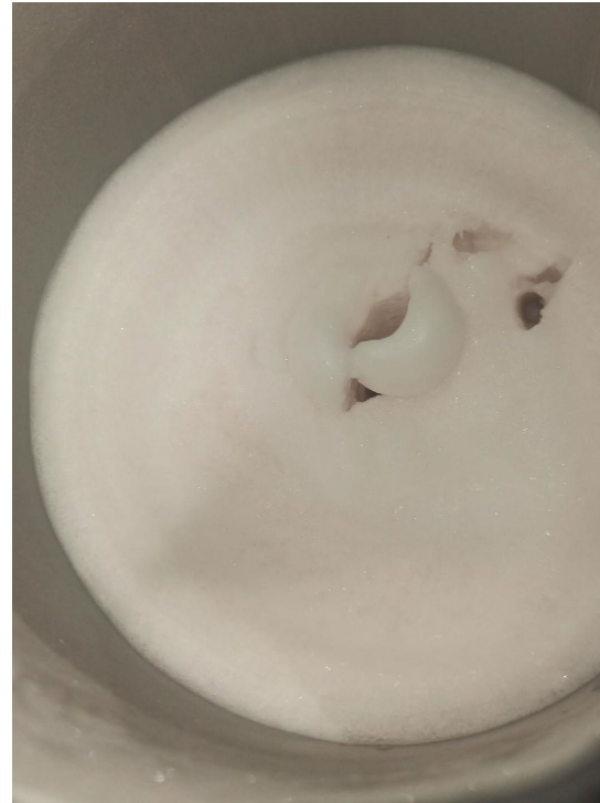
Figure 7.8. Structure of formed ice from studied brine solution when the salt concentration is low in S5 (A), and when the concentration of ice is high in S1 (B).
