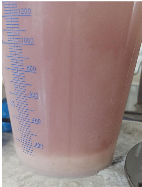
Figure 7.12. First trials of salt crystallization using PFC on brine solutions from meat processing industry.
