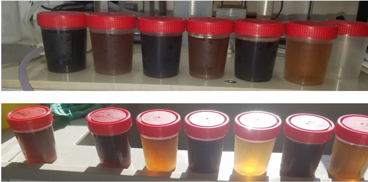
Figure 5.7. Raw RO concentrate of reverse osmosis, the concentrated and the ice fractions generated through the PFC and SFC in two stages.
