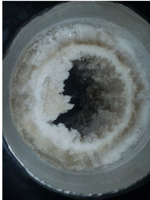
Figure 5.4. Formed ice in the PFC of the RO concentrate, A) before and B) after vacuum application.
