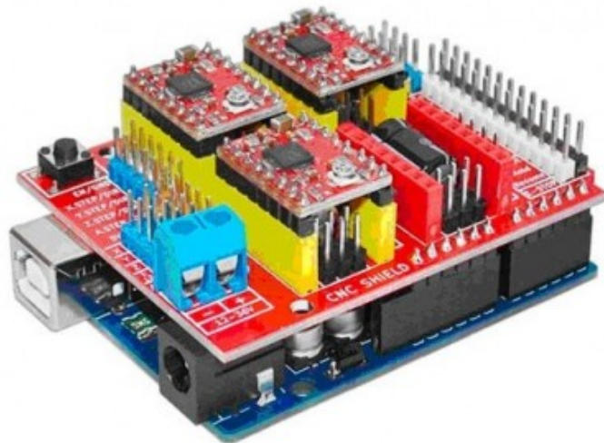
Figure 18: CB assembly (Arduino UNO with CNC Shield and motor drivers).
