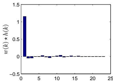
Fig. 5. The coefficients of the global filter  $w(k) \star h(k)$ .
