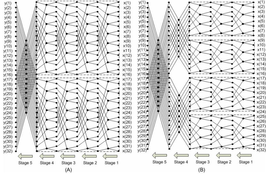
**Figure 2** A 32-point radix-2 stage-to-stage interconnection pattern representations for the required new first family of solutions. Case A) with parameter  $a=1$ : one Cooley-Tukey type stage and two blocks with regular interconnection pattern. Case B) with parameter  $a=2$ : two Cooley-Tukey type stages and four blocks with regular interconnection pattern.
