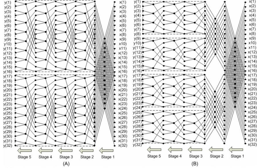
**Figure 3** A 32-point radix-2 stage-to-stage interconnection pattern representations for the required new second family of solutions. Case A) with parameter  $a=1$ : one Cooley-Tukey type stage and two blocks with regular interconnection pattern. Case B) with parameter  $a=2$ : two Cooley-Tukey type stages and four blocks with regular interconnection pattern.
