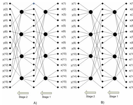
**Figure 4** A 16-point radix-4 equal interconnection pattern stage-to-stage solutions obtained from A) the first family of solutions and B) the second family of solutions, both for parameter  $a=0$ . These two solutions have 0 Cooley-Tokey type stages and only 1 block exhibiting the same interconnection pattern and they are the same as the radix-4Pease solutions.
