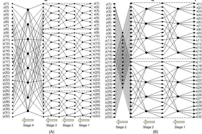
**Figure 5** 32-point FFT mixed-radix factorizations combining (A) 1 radix-4 stage with 4 subblocks with 3 radix-2 equal interconnection pattern stages and (B) 1 radix-2 stage with 2 subblocks with 2 radix-4 equal
