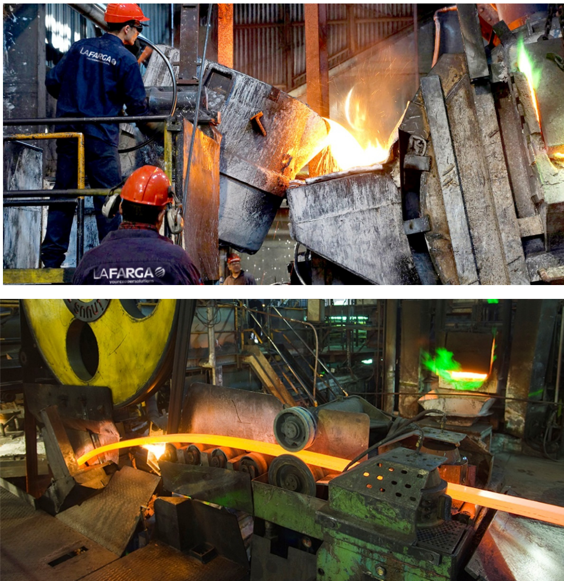
Figure 2. Stages of the process of manufacturing wire rods.
