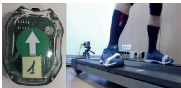
Figure 1. Left: Image of the sensor used in this study. Right: Initial position of the participant on the running treadmill, with the sensor fixed on the footwear. Author's source.
